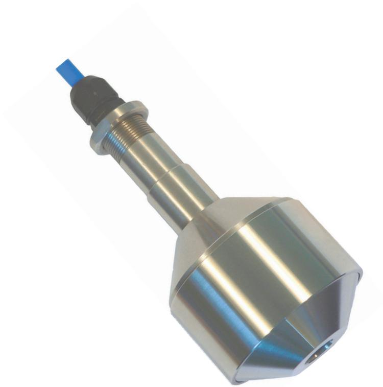
The OxyGuard probe is a membrane covered galvanic cell that generates an electrical signal proportional to the oxygen pressure it senses, no matter which medium it is placed in.
